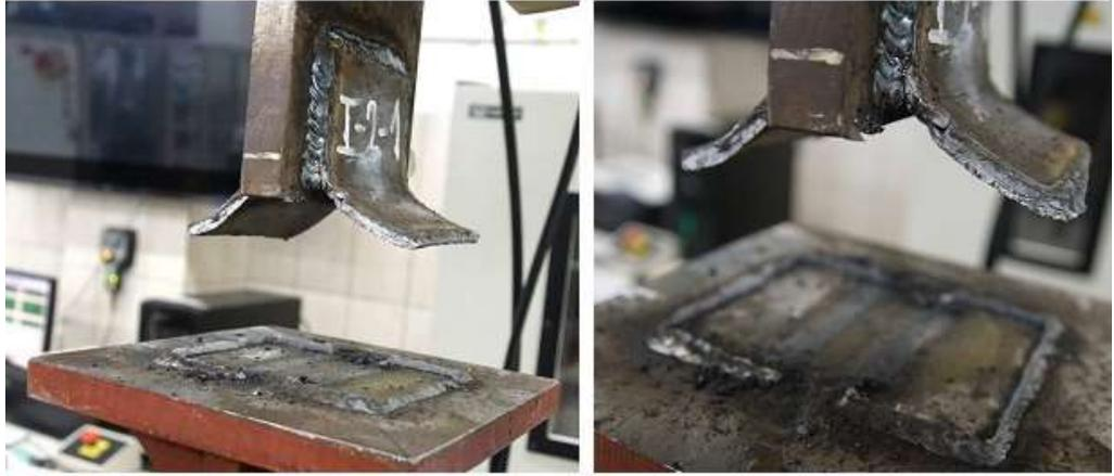
**Разрушение образца I-2-2**
